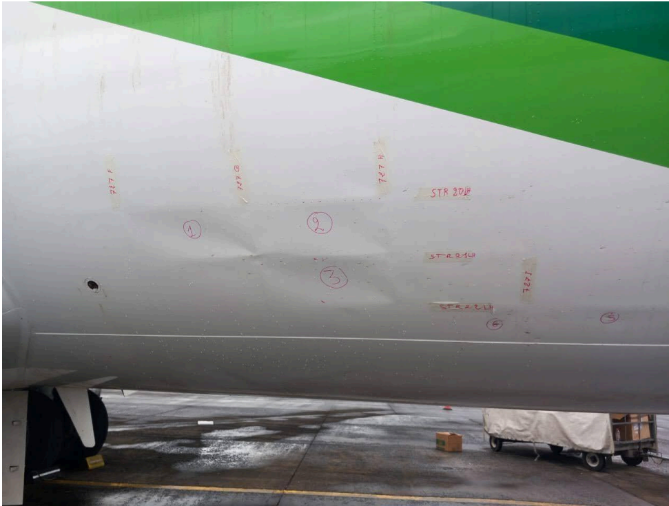
Figure 5: Damage to left side fuselage skin
