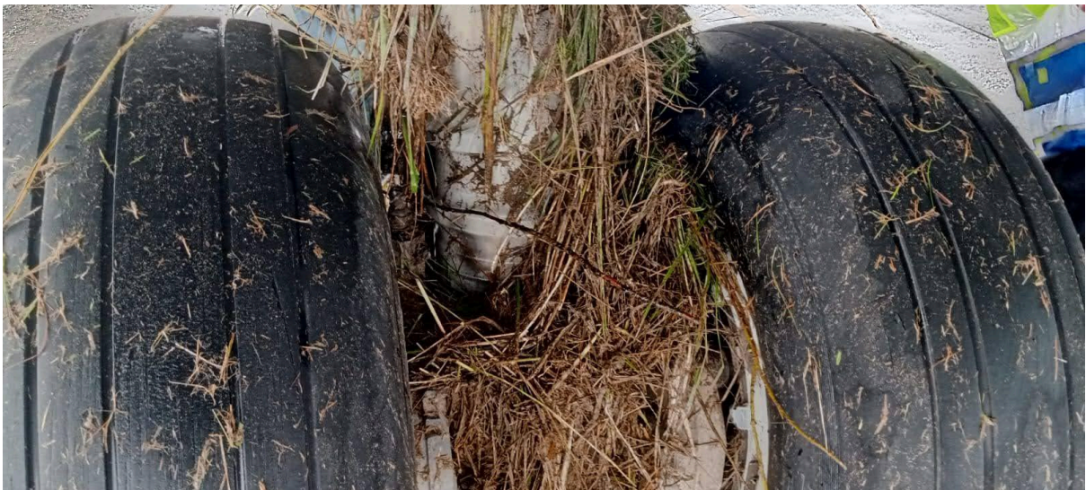
Figure 4: Debris on left landing gear strut
