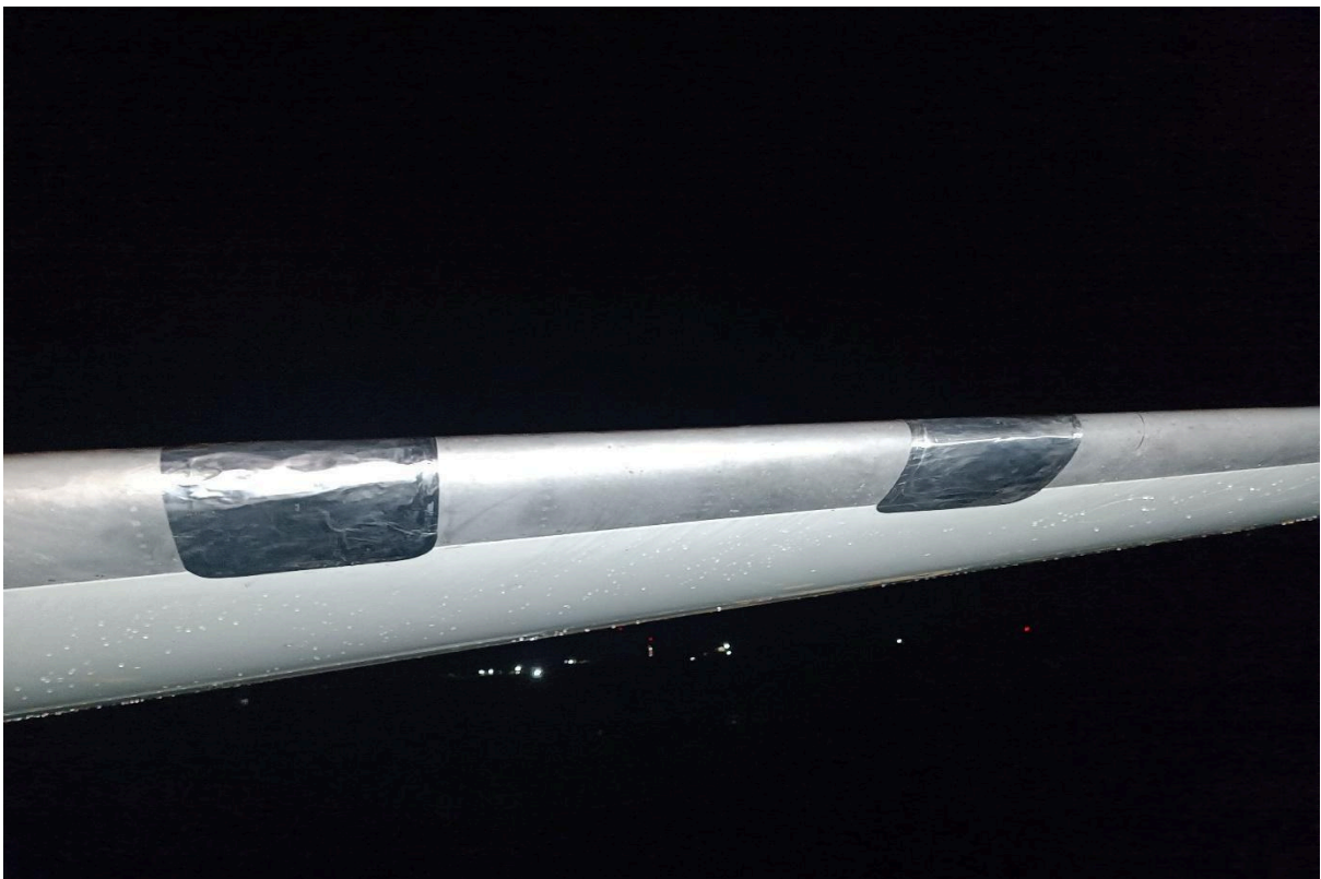
Figure 6: Dent on the left hand horizontal stabilizer leading edge skin with speed tape
