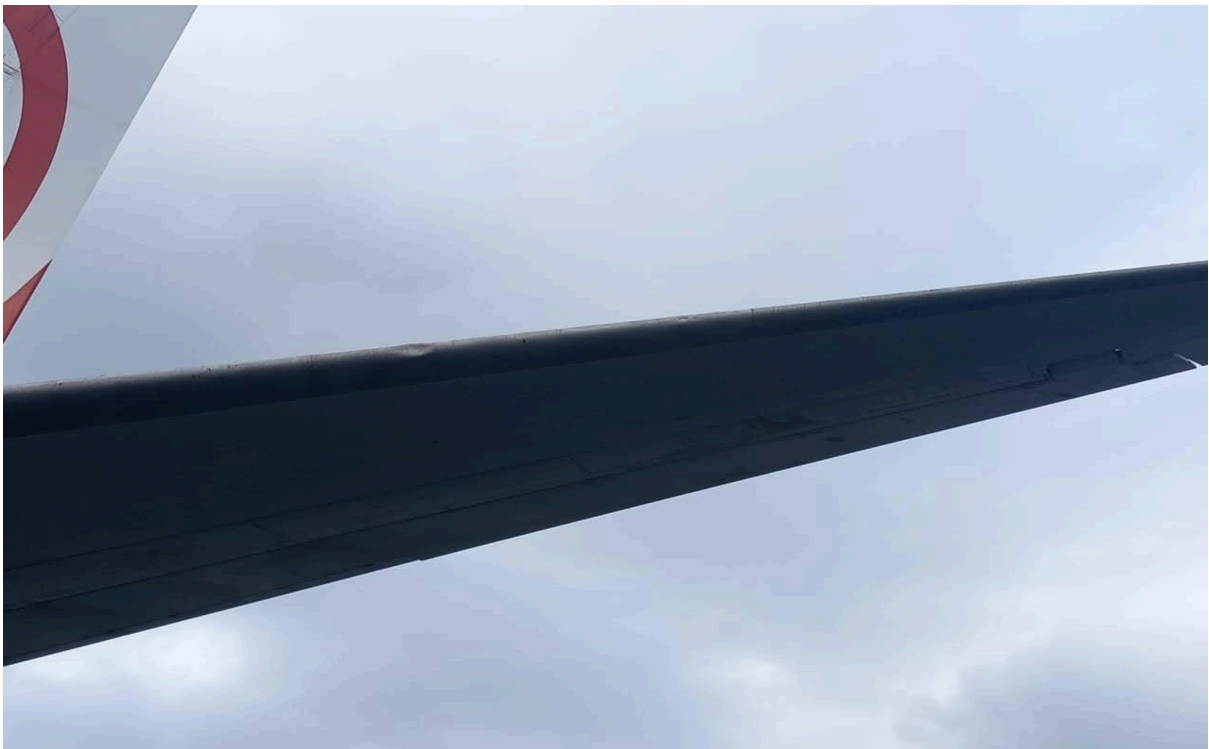
Figure 8: Dent created on the left hand horizontal stabilizer leading edge skin
