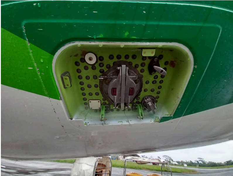
Figure 1: A view of the lavatory compartment with missing panel cover
