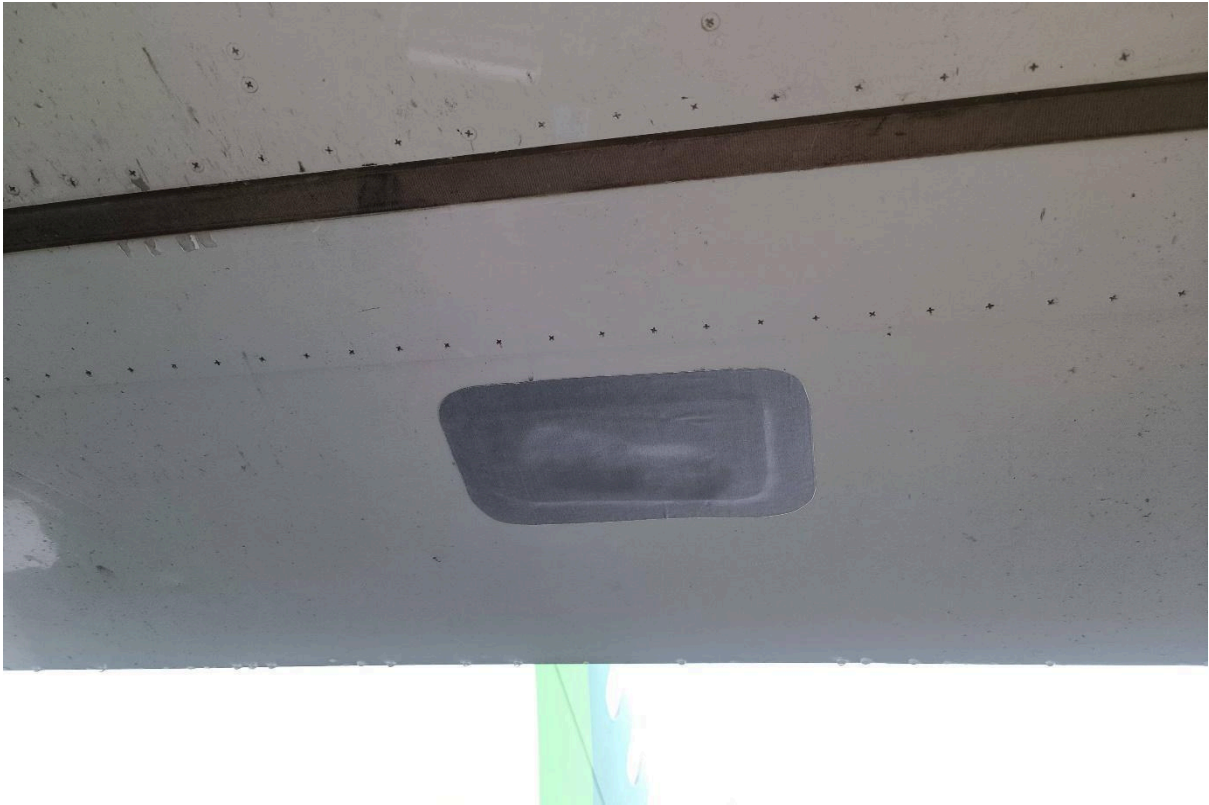
Figure 7: Crack to left hand wing inboard aft flap lower skin covered by speed tape
