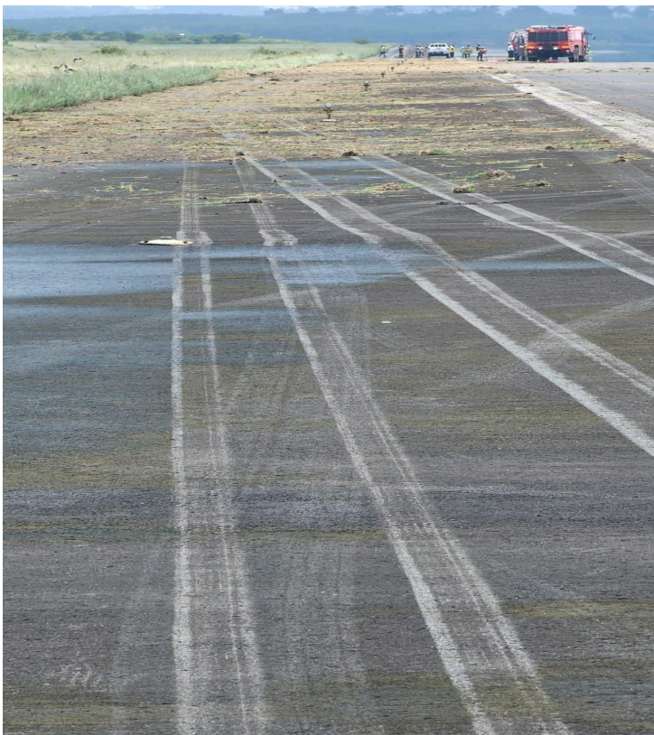
Figure 2: A view of Runway 04 left shoulder showing the aircraft tire tracks leaving the runway
