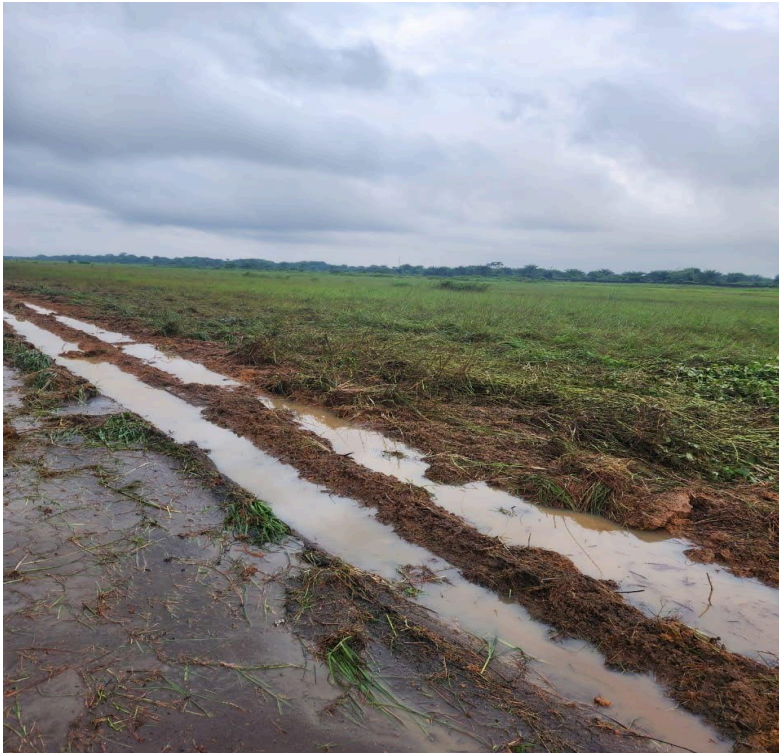
Figure 3: View of rut created by left two tires of the left landing gear on edge of runway 04
