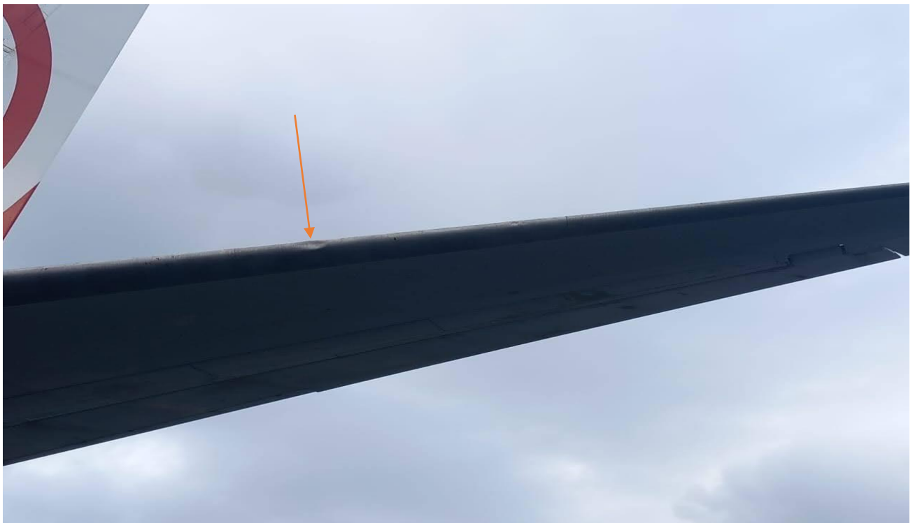
Figure 14. Dent created on the left-hand horizontal stabilizer leading edge skin
