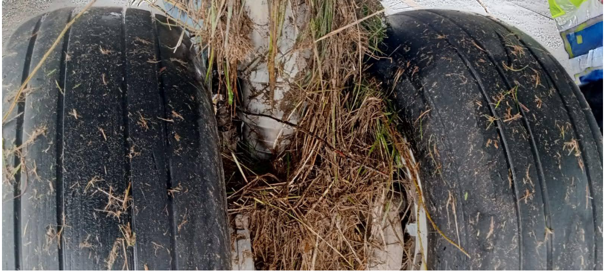
Figure 11. Debris on left main landing gear strut
