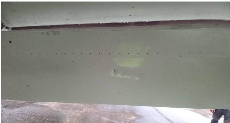
Figure 16. Dent with crack to the AFT flap lower skin
