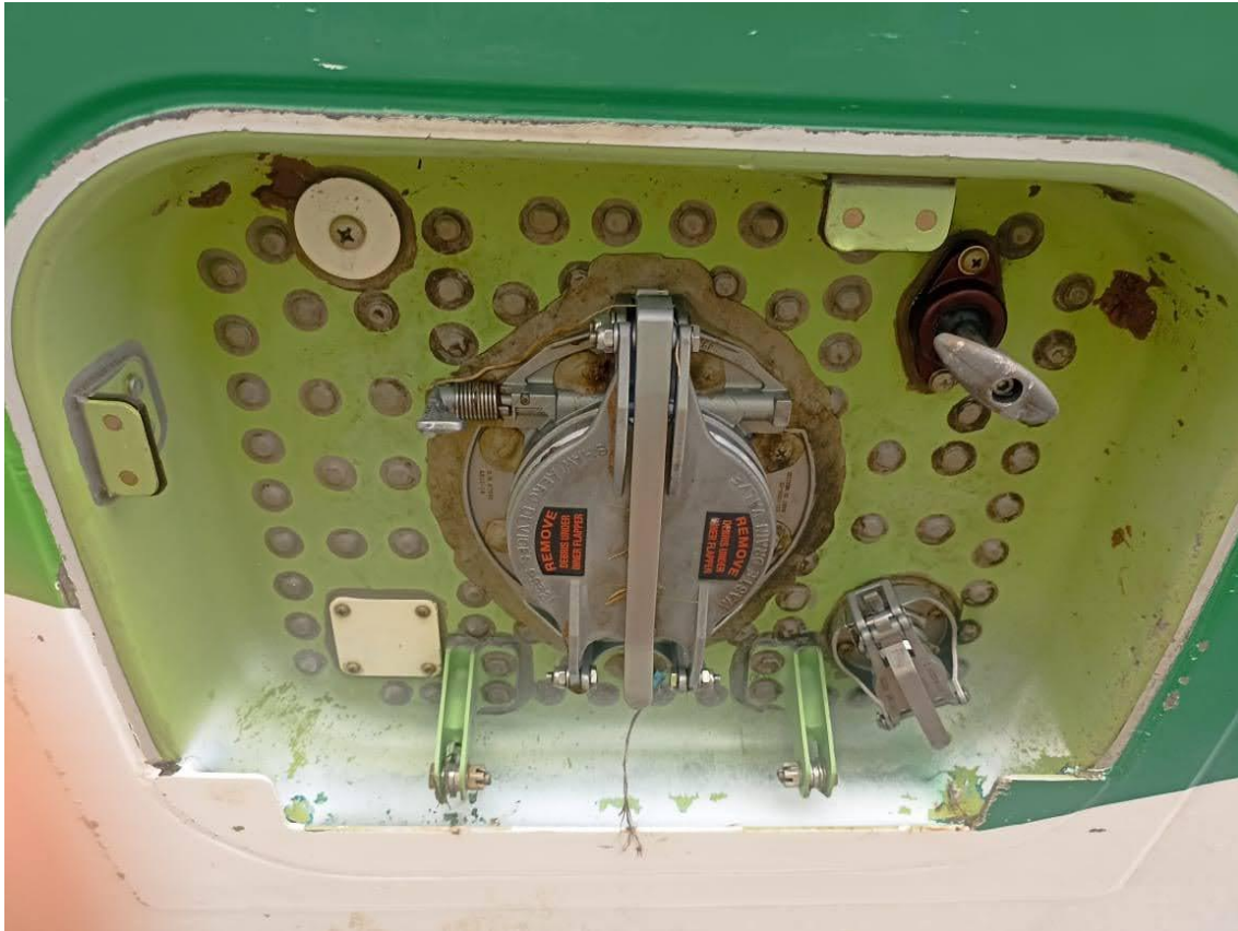
Figure 15. Lavatory service panel without cover
