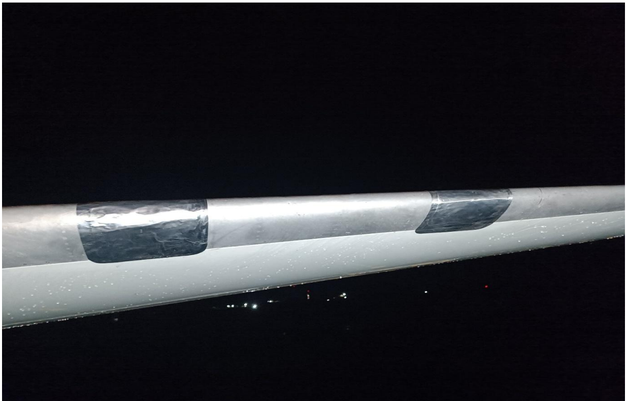
Figure 12. Speed tape on the dent mark of the left-hand horizontal stabilizer leading edge skin
