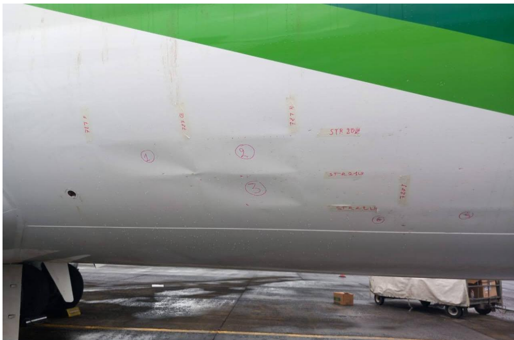
Figure 10. Damage to left side fuselage skin
