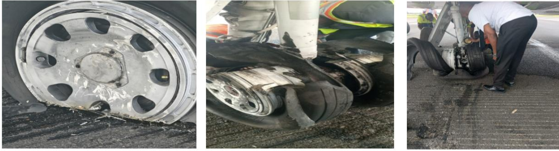
Figure 5: Left main landing gear initial damage post-occurrence
