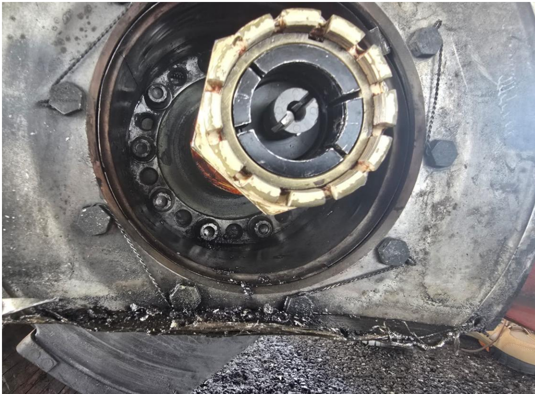
Image 4: View of the ant-skid unit prior to replacement
