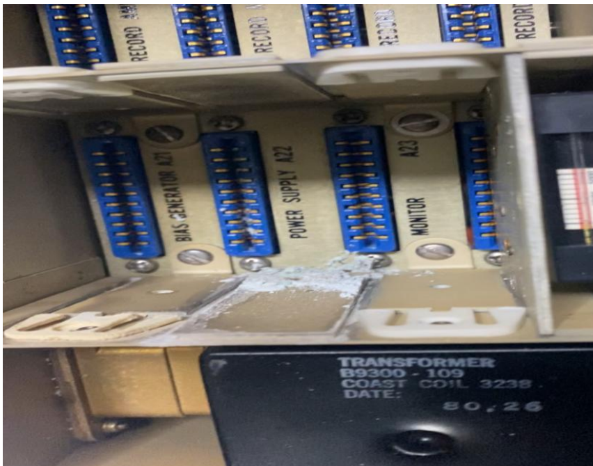
Image 8: Signs of Corrosion in the chip housing
