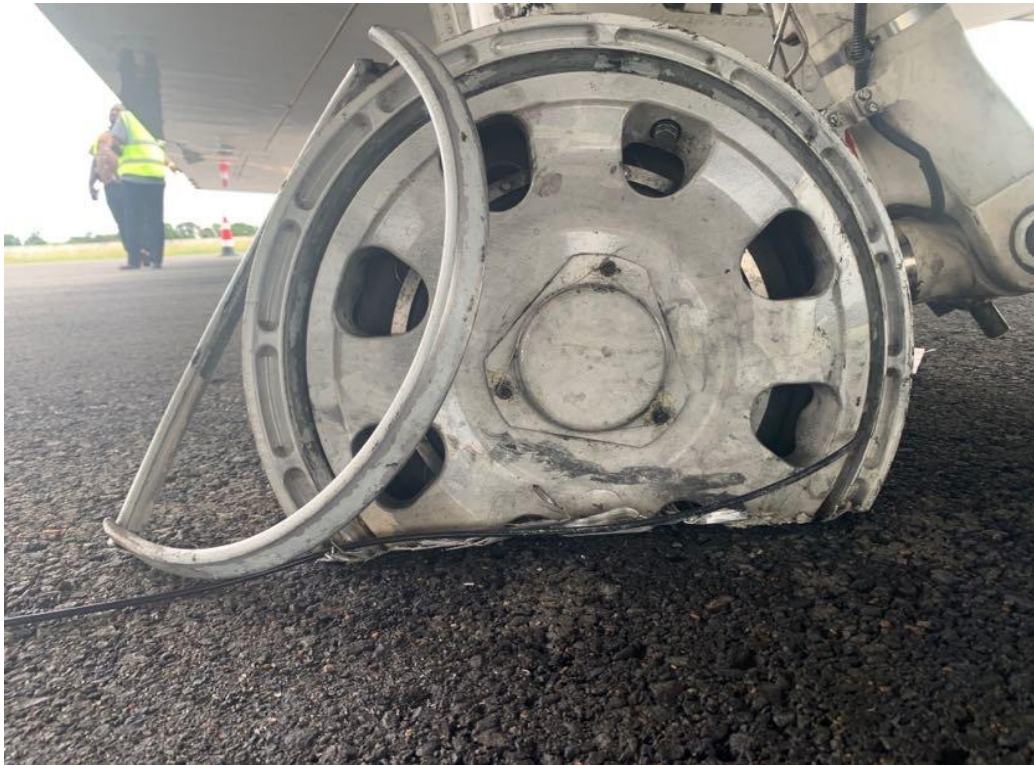
Figure 6: Secondary damage sustained as a result of removal of disabled aircraft
