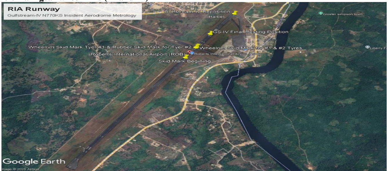
Figure 2: View of the coordinates and distances of skid marks points, final resting position, and repositioned point.
