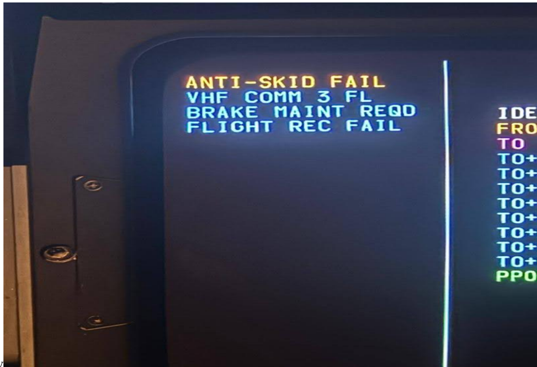
Image 6: Annunciator panel highlighting anti-skid fail in amber
