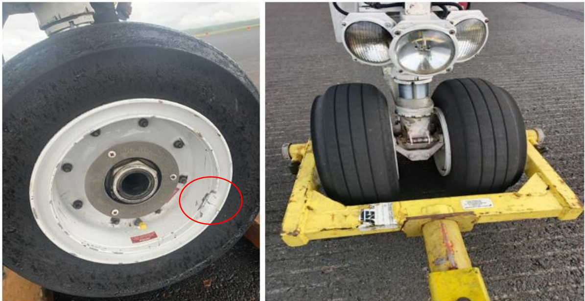
Figure 4: Damage caused to the right nose wheel by the tow bar
