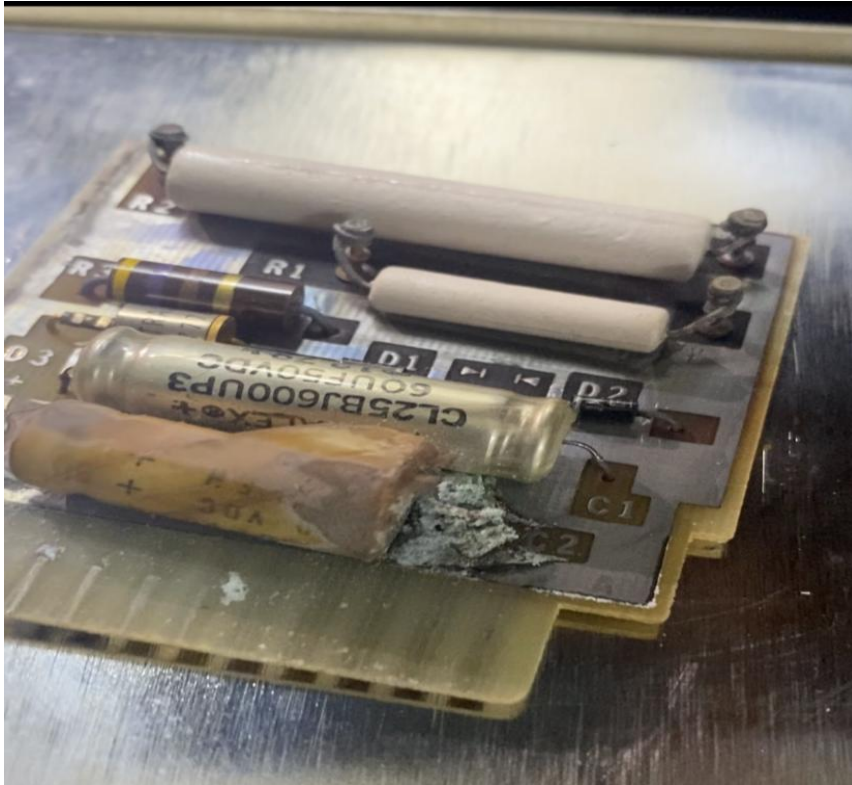
Image 7: Corroded Power supply chip of the CVR after retrieval
