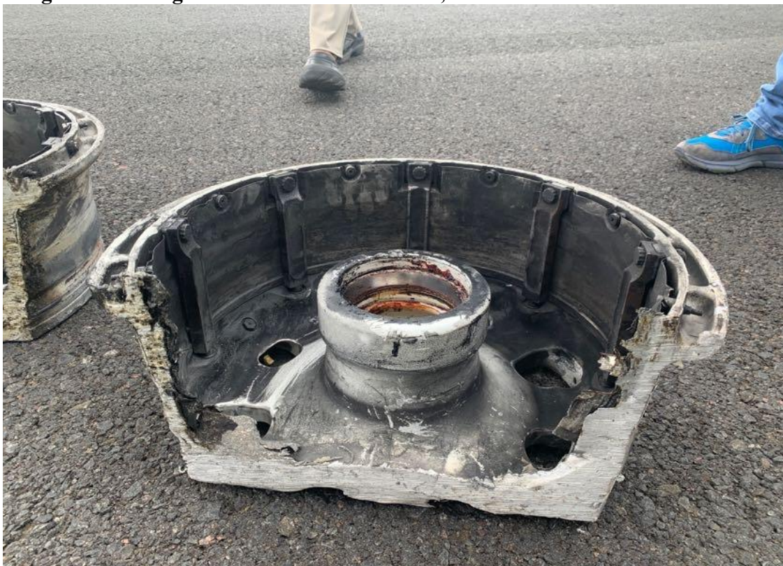
Image 2: A view of the deformed wheel
